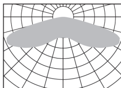
LS12 ME600 Lighting for one or two-sided arrangement of poles, also with lower mounting heights and larger distances
